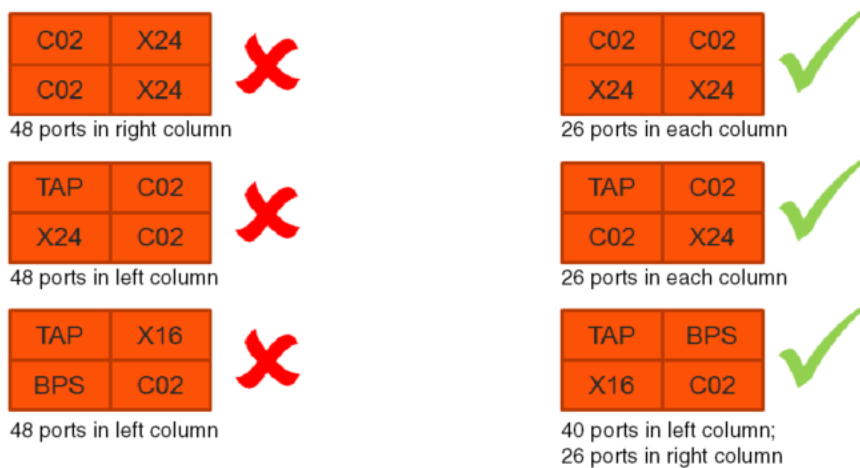
Figure 7 Module Placement of PRT-HC0-CO2, 100G Mode
